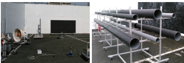
Fig. 1 Experimental imaging system for gas leak (left) and simulated piping equipment (right).
